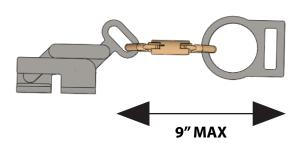
When connecting to the ladder system, do not use any connector that will allow a distance of more than 9" from your front D-Ring to the cable grab. Guardian strongly reccomends the use os a 01813-S carabineer as shown in the picture to the left.
