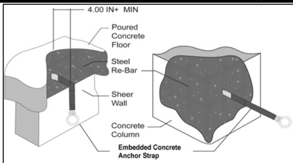
This anchor is part of a comprehensive PFAS or PRS. It must be used in conjunction with a Full Body Harness with back D-ring and a Shock Absorbing Lanyard/Self-Retracting Lifeline that limits freefall to 6 feet or less. When used as a component of a PRS, it must be used with a Full Body Harness or Work Positioning Belt and a Positioning Lanyard.
