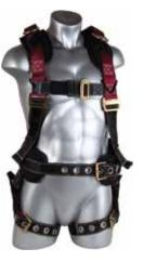
**Personal Fall Arrest:** Seraph Harness may be used in Personal Fall Arrest applications as a component of a Personal Fall Arrest System (PFAS). Structure must withstand loads applied in the directions permitted by the system of at least 5,000 lbs. Maximum free fall is 6', unless used in combination with equipment explicitly certified for extended free fall. Applicable D-ring: Dorsal.
