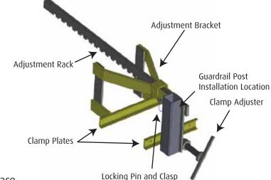
For use in combination with Universal Guardrail Post (part #: 61133, 61135, or 61136) and 2" x 4" OR 2" x 6" construction grade lumber guardrails. Guardrails must overlap at least 12" at each end.
