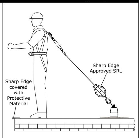
**1 Certified Anchorage:** An anchorage for Fall Arrest, Positioning, Restraint, or Rescue systems that a Qualified Person certifies to be capable of supporting the potential fall forces that could be encountered during a fall or that meet the criteria for a certified anchorage prescribed in the ANSI Z359 standards.
