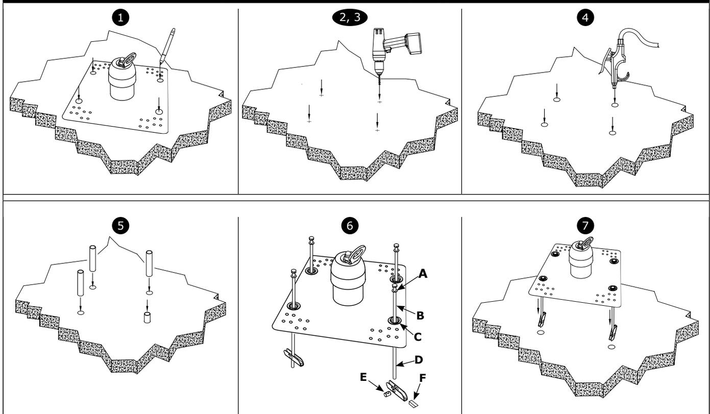
4. Insert an air nozzle in each mounting hole and blow out any debris with an air pump or low-pressure compressed air (Figure 10-4).
