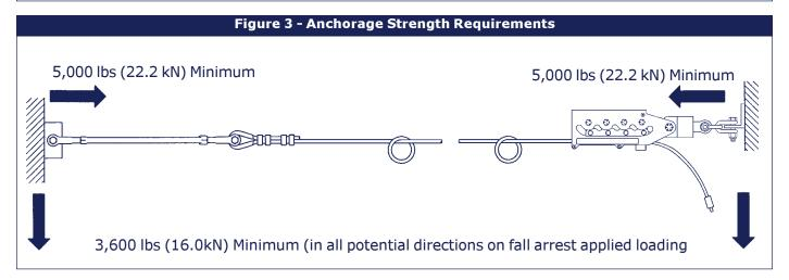
**2.5 CONNECTING SUBSYSTEM:** The connecting subsystem is the portion of the personal fall arrest system that is used to connect between the horizontal lifeline subsystem and harness fall arrest attachment element. The connecting subsystem must limit forces applied to the horizontal lifeline to 900 lbs. or less.
