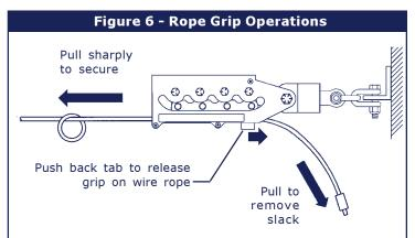
**Step 4:** If slack is needed to make an adjustment to the system, or for ease in removing the system, press back toward the anchor on the release tab on the bottom of the cable grip device as shown in Figure 6. After the lifeline has been tensioned, it may be necessary to tap the release tab with a hammer to disengage the cable grip device from the lifeline.
